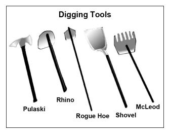
Pulaski – for loosening and scraping dirt and chopping roots along the trail bed
